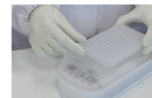
Once the 96 wells plate is full, remove the holder and place it in the decoding platform which is connected to the PCR instrument for amplification
