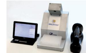
Copan MALDItrace™ is a system for the traceability of biological sample spotted into a 96 well plate for DNA quantification (PCR) or DNA sequencing
