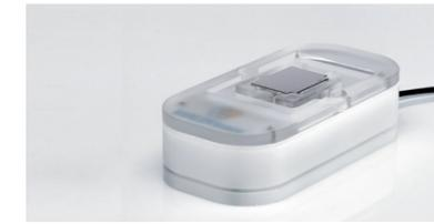
Once the target plate is full or panel of tests completed, remove the RFID Embedded Target Plate Holder from the MALDI-Trace® Workstation and
