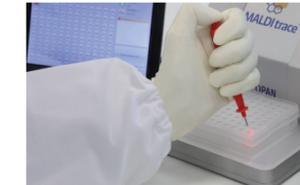
Spot the punch into the illuminated target well
