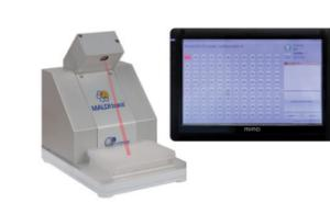
The MALDItrace™ software automatically designates the well location using the laser designator. The RFID chip automatically logs location of the test ID
