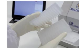
Place the 96 wells plate into the Plexiglass holder and place the holder onto the MALDItrace™ workstation
