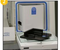
Transfer all system components into the workstation through the airlock. Transfer is shown in two stages through a small Whitley airlock. All parts can be transferred simultaneously in a large Whitley airlock.
