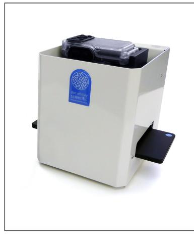
The Whitley Petrifoto System consists of a compact digital camera, camera adaptor, battery and battery charger, microSDHC card and adapter, light box, power supply and a Petri dish holder. Ensure the camera is outside the workstation when changing the battery or memory cards. A storage case for spare cards is also supplied.
