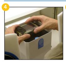
Place the camera onto the camera adaptor. Place a Petri dish in the Petri dish holder.
